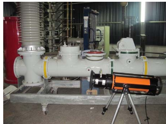
Fig. 5 X-ray machine and the imaging plate
