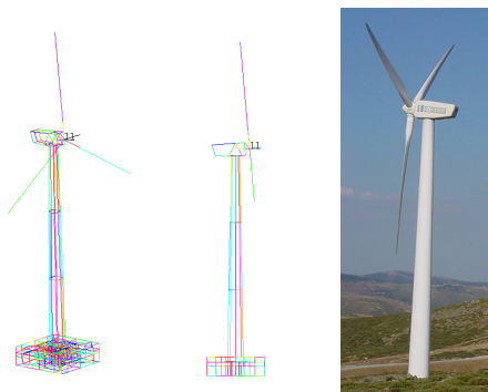
Fig. 3 Wireframe model and photo of the wind turbine MADE AE-46/1
