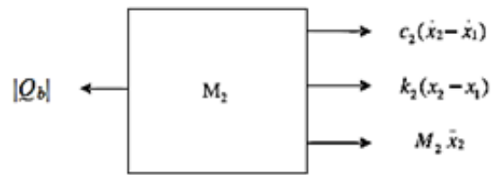
Fig. 4 Magnitude of Dynamic Earth Thrust
