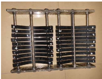
Fig. 1 Bending fixture for CFRP plates
