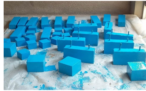
Fig. 2 Epoxy coating for the concrete specimens
