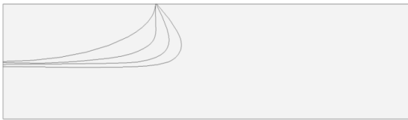
Fig. 10 Crack shape sequence for a deep semi-elliptical surface crack under bending ( a/w=0.5 , a/c=0.33 )
