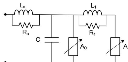
Fig. 6 IEEE frequency-dependent model
