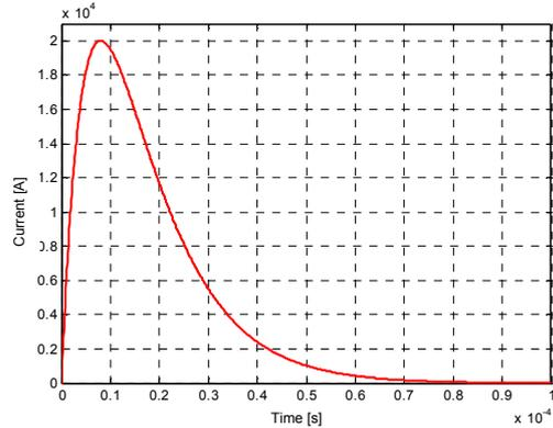
Fig. 11 Discharge current 20kA with impulsive form 8/20µs/µs
