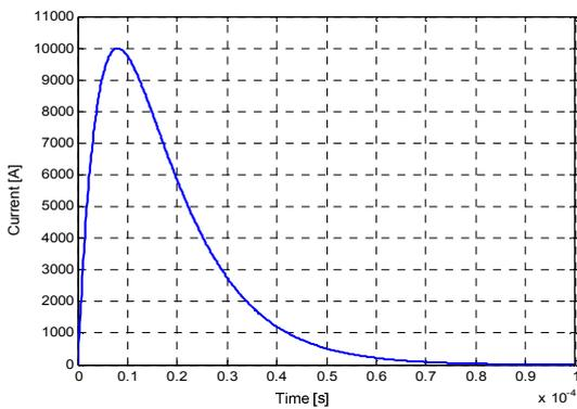
Fig. 9 Discharge current 10kA with impulsive form 8/20µs/µs
