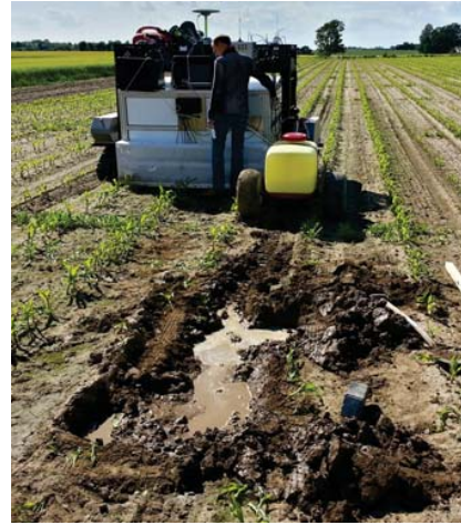
Fig. 1 The remains of a parcel in which the tool carrier was stuck during spraying
