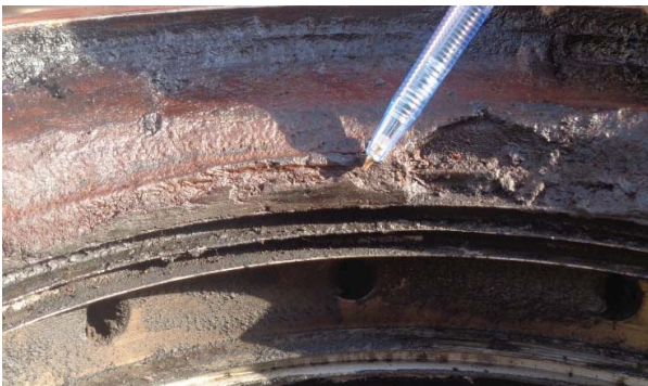
Fig. 13 Shedding of coke deposits after getting rubbed
