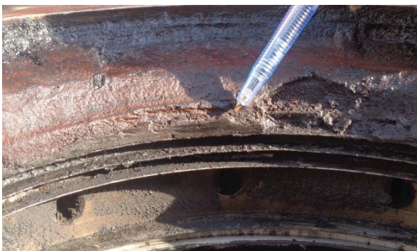
Fig. 13 Shedding of coke deposits after getting rubbed
