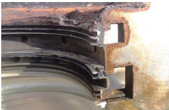
Fig. 12 Physical texture of Coke puddles
