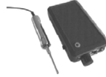
Fig. 6 Vibration sensor unit and amplifier
