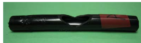
Fig. 1 Cross section deformation spring (CSDS)
