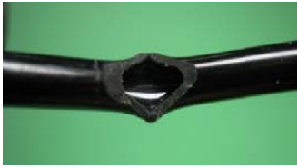
Fig. 2 Deformation of the CSDS during bending
