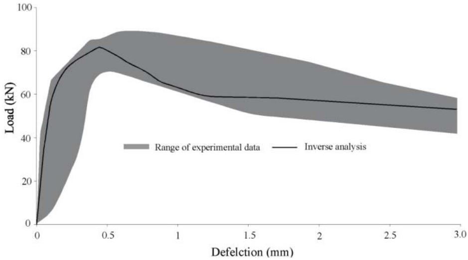
Fig. 10 Measured and calculated P- $\delta$  behaviors: Proposed  $\sigma$ - $\epsilon$  relationship-HSFR-90
