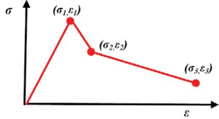
Fig. 12 The shape of tensile  $\sigma$ - $\epsilon$  relationship
