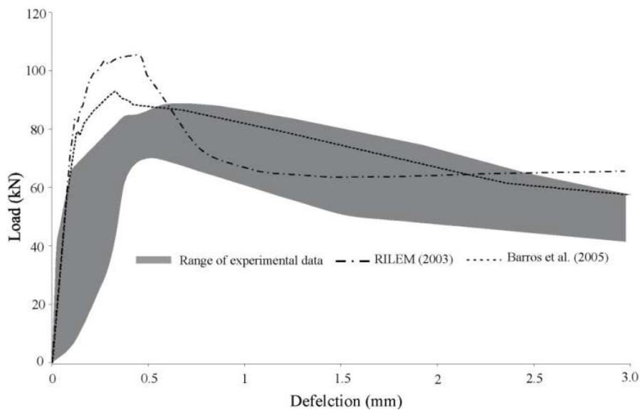
Fig. 6 Measured and calculated P- $\delta$  behaviors: First estimate  $\sigma$ - $\varepsilon$  relationship-HSFRC-90
