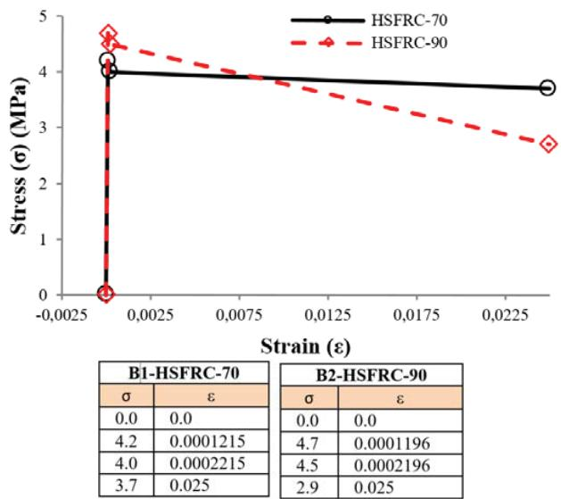
Fig. 8 Proposed tensile  $\sigma$ - $\epsilon$  relationships for HSFRC beams were adapted in NLFEA
