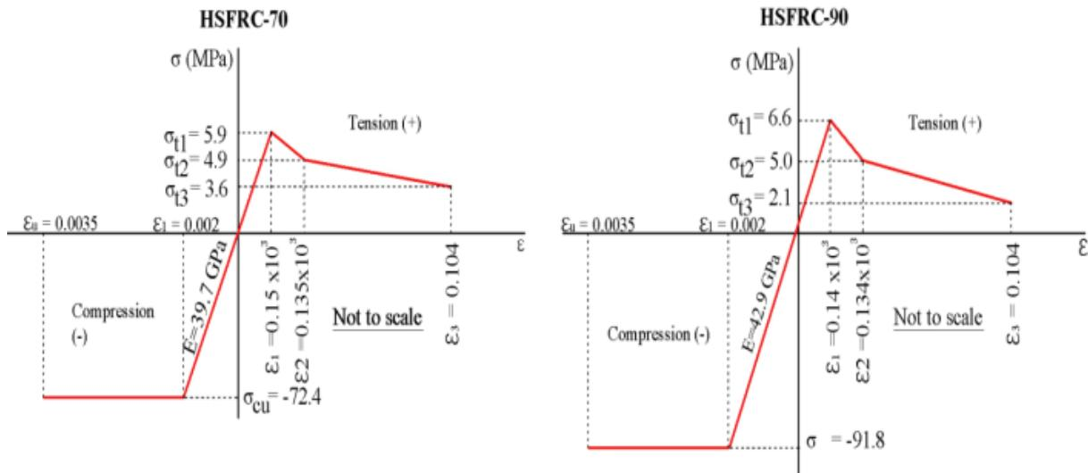
Fig. 4 The first estimate of the  $\sigma$ - $\varepsilon$  relationship for HSFRC according to [3]
