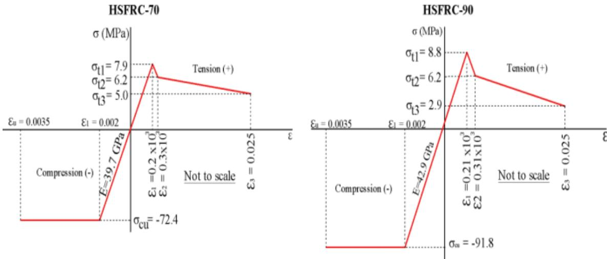
Fig. 3 The first estimate of the  $\sigma$ - $\varepsilon$  relationship for HSFRC according to RILEM, [2]
