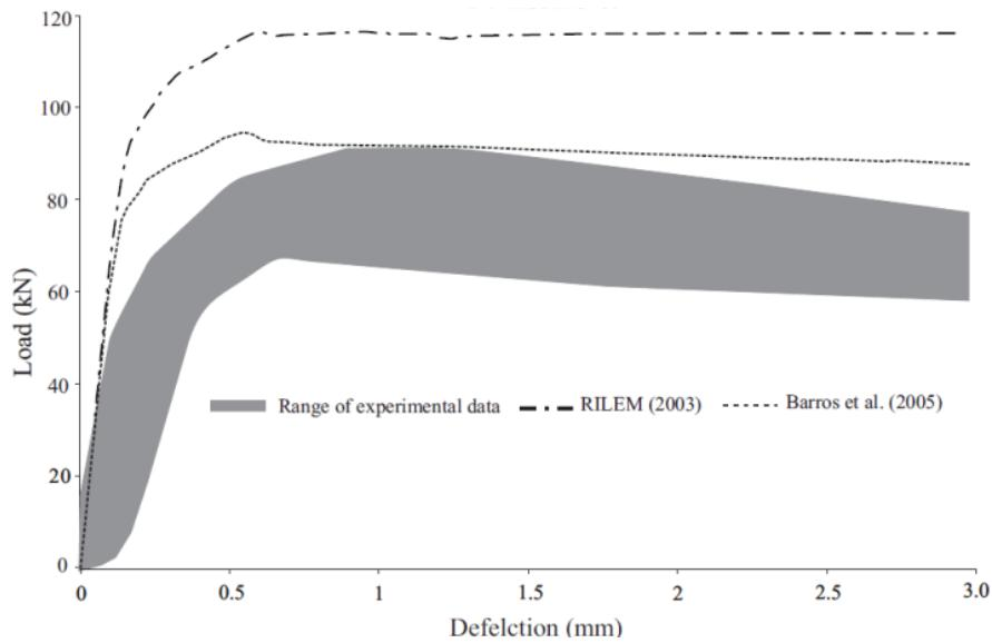
Fig. 5 Measured and calculated P- $\delta$  behaviors: First estimate  $\sigma$ - $\varepsilon$  relationship-HSFRC-70
