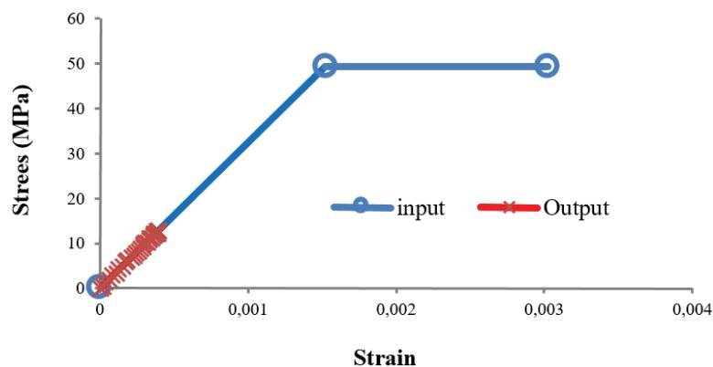
Fig. 7 Proposed input and output compressive  $\sigma$ - $\varepsilon$  relationship
