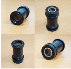
Fig. 2 Optical system of star tracker experimental model
