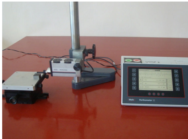
Fig. 2 Perthometer for measurement the surface roughness of the sample
