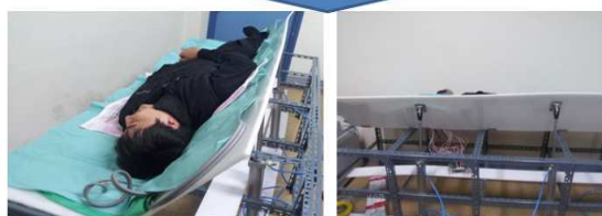
Fig. 4 Position change using air cylinder
