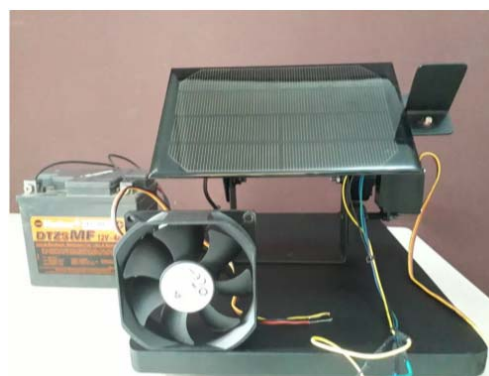
Fig. 3 Solar tracker for photovoltaic panels with didactic applications
