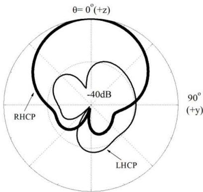
Fig. 4 Measured radiation pattern of microstrip patch
