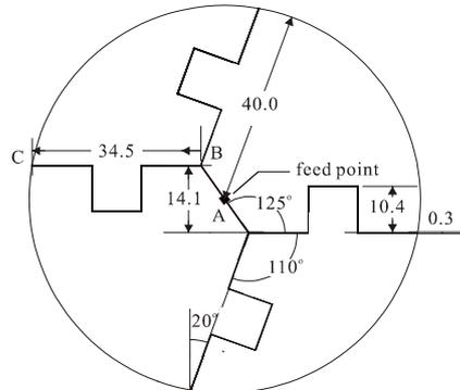
Fig. 10 Design of feed network of  $1 \times 4$  array.
