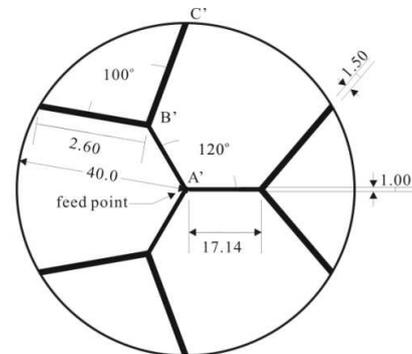
Fig. 11 Design of feed network of  $1 \times 6$  array.
