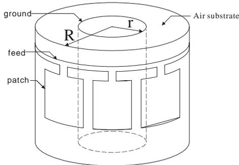
Fig. 8 Design of low-profile omni-directional antenna on UAV.
