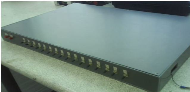
Fig. 9 Photographic view of the developed AWG-based OCDMA encode prototype (Front view)
