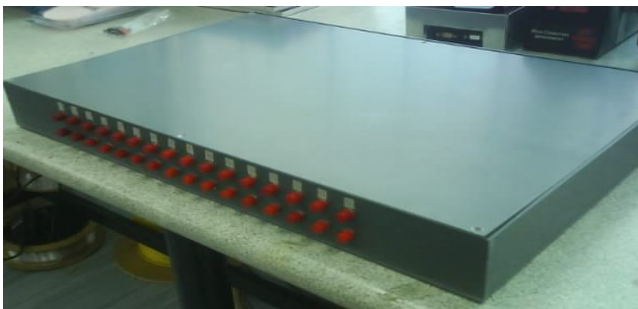
Fig. 10 Photographic view of the developed AWG-based OCDMA encode prototype (Back view)
