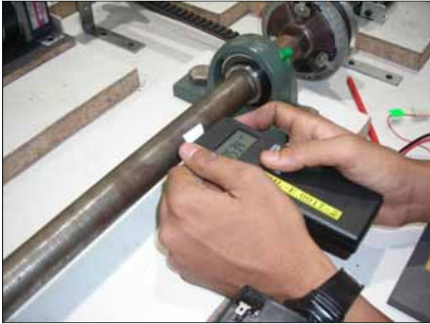
Fig. 4 Using of tachometer to obtain shaft speed
