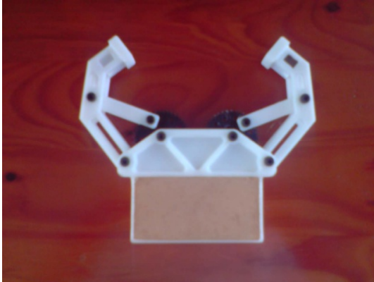
Fig. 2 The final gripper that has been design with SolidWorks and rapidly manufactured by using 3D printing method
