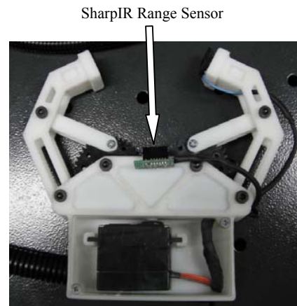
Fig. 5 Placement of range sensor and FSR on the gripper
