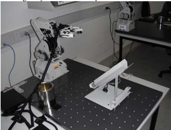
Fig. 7 Lab Volt 5150 robot with mounted gripper setup
