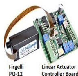
Fig. 4 Firgelli PQ-12 linear actuator and controller board
