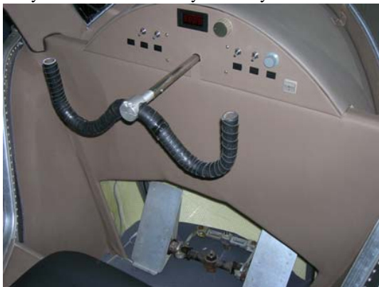
Fig. 6 Real cockpit with control loading system
