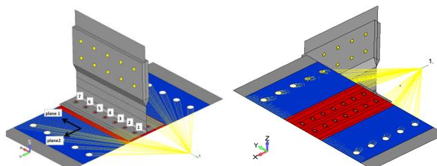
Fig. 7 Boundary condition for shear test simulation
