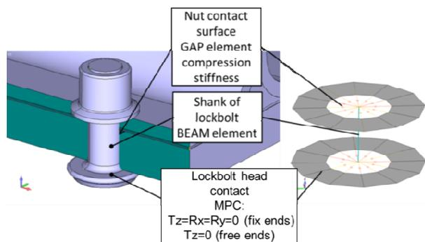
Fig. 6 Description of rivet discretization by FE elements
