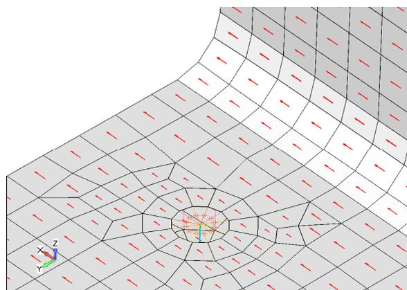
Fig. 3 Material coordinate system in shell elements
