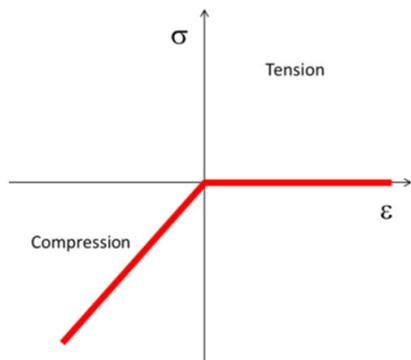
Fig. 5 Property of GAP elements for contact simulation
