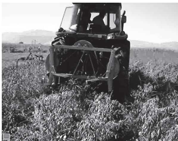
Fig. 11 Harvest experiments with prototype pepper harvest machine
