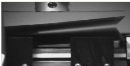
Fig. 7 Wafer lifting during picking process
