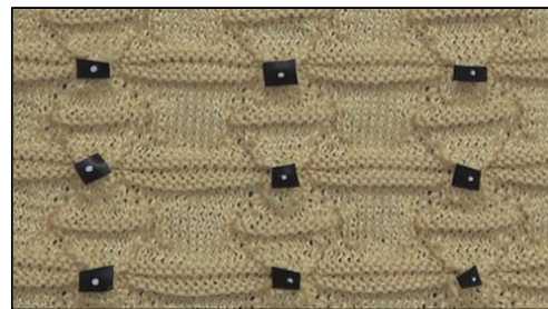
Fig. 7 Marked points in the fabrics to measure the distance between them
