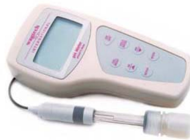
Fig. 3 Sample of a hand held probe to conduct daily tests at the sewage facility
