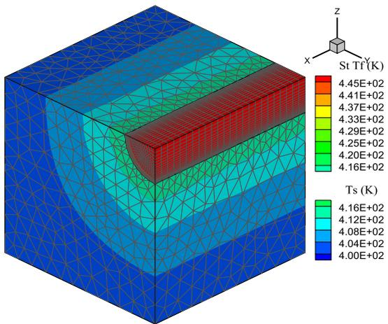
Fig. 9a 3D view of the 2D case conjugate system showing the meshes and the colour bands of temperature in both domains
