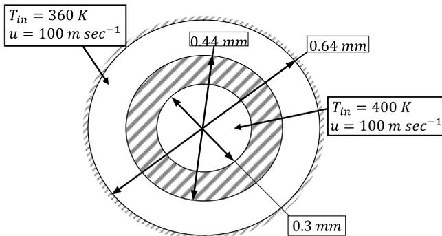
Fig. 7 An approximate dimension scale of the concurrent heat exchanger
