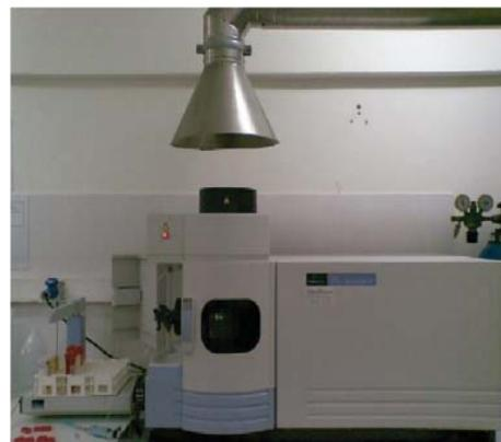
Fig. 4 Perkin-Elmer Optima 2100 DV, ICP-OES
