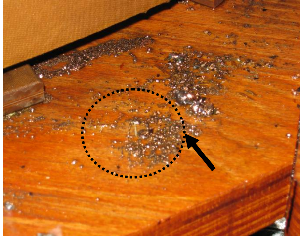
Fig. 11: Eroded copper chips
