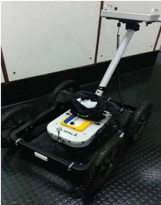
Fig. 1 GPR on a Terraplug Rough Terrain Cart
