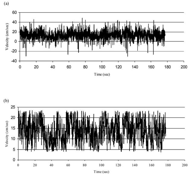
Fig. 2 Vectrino data (a) before spike removal (b) after spike removal
