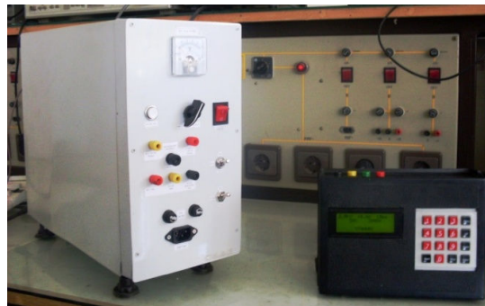
Fig. 3 Electrical and Controller unit of PEF set
