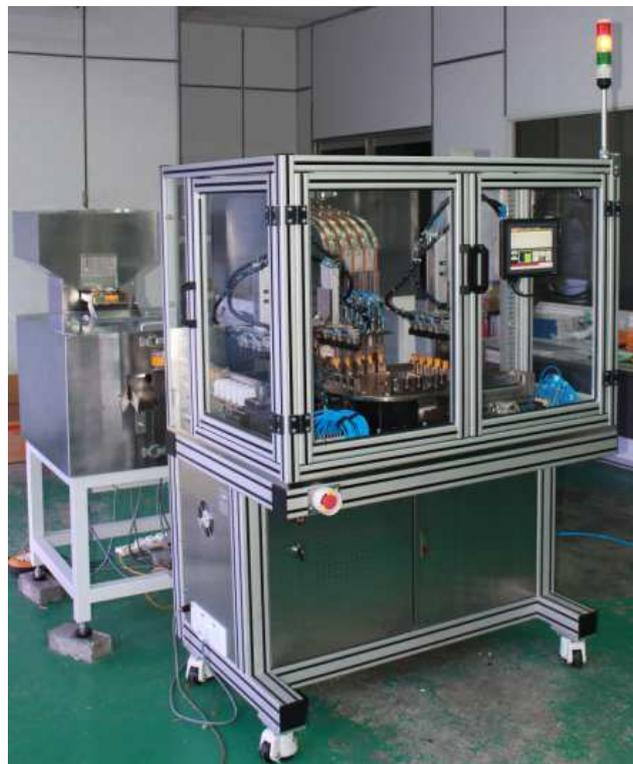
Fig. 20 Roller clamp robotic assembly system
