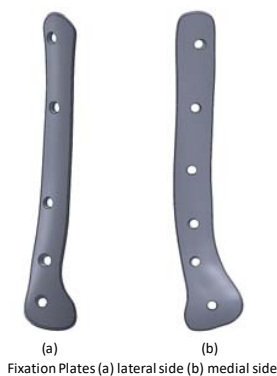
Fig. 3 Customized implant designed for fractured bone
