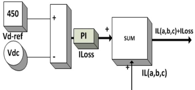
Fig. 1 FA Control method, giving back Iloss current to the system
