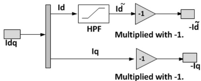
Fig. 4 Obtaining AC current component of  $I_d$
