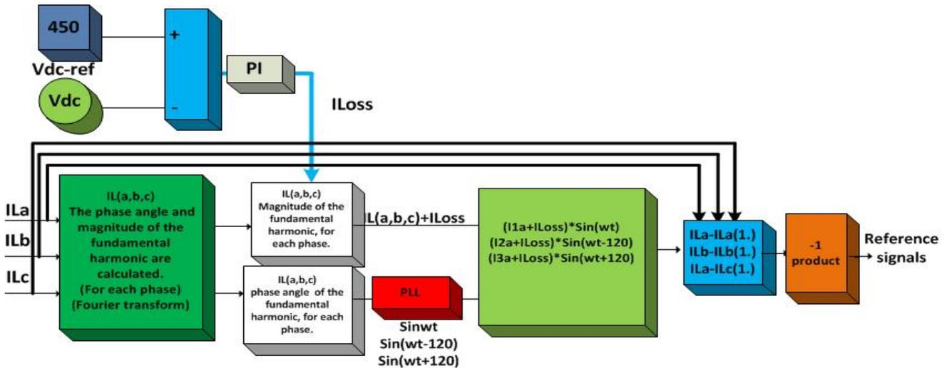
Fig. 3 General algorithm of FA control method
