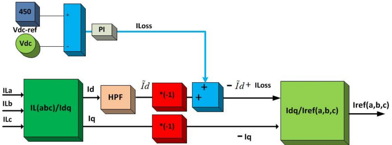
Fig. 5 General algorithm of SRF control method
