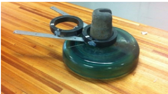
Fig. 10 Adapted prototype LC sensor with its mechanical clamps around a glass insulator
