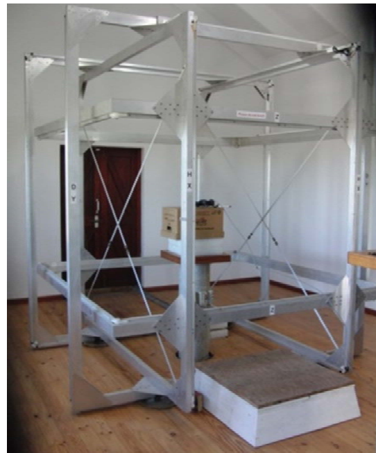
Fig. 11 3-axis Helmholtz coil system for calibration of the prototype LC sensor
