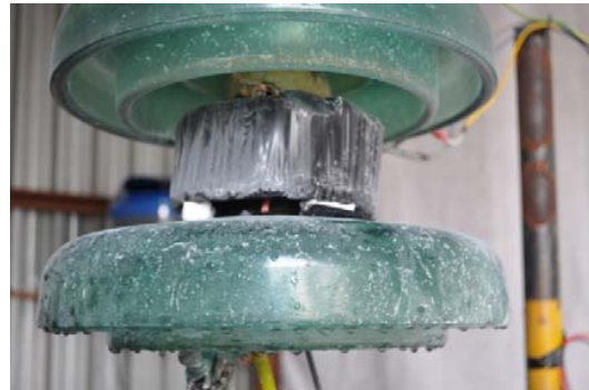
Fig. 8 LC test setup showing the pollution on the outside of prototype and insulators (with two stand-off insulators)
