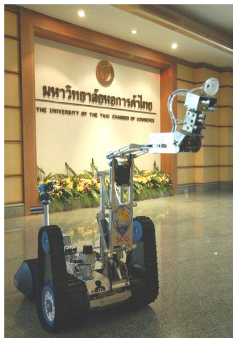
Fig. 1 CEO Mission II rescue robot with 5-Joint mechanical arm
