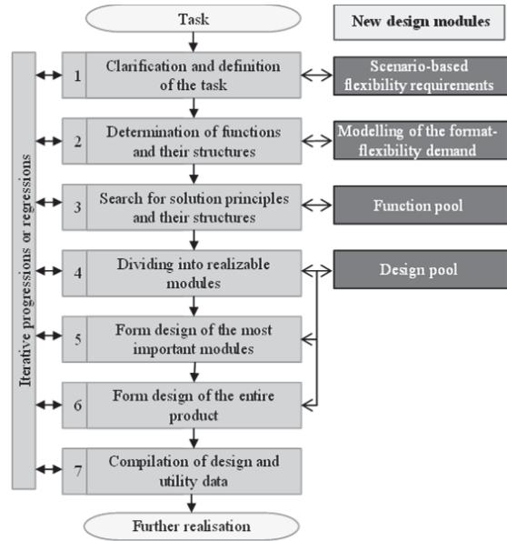
Fig. 9 Design-led approach integrated in the VDI-2221
