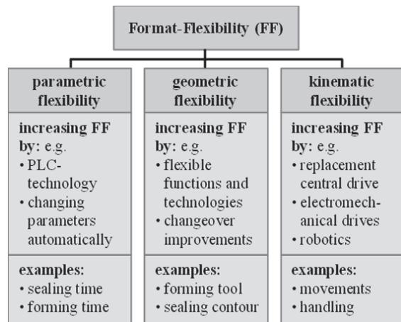
Fig. 2 Classification of enabler for increasing format-flexibility
