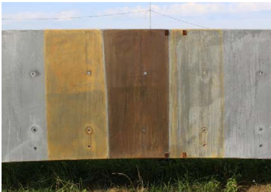
Fig. 23 Surface after acid treatment
