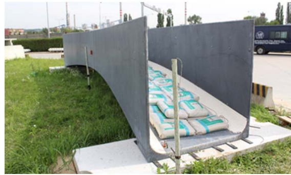
Fig. 19 Perform static loading test on footbridge II
