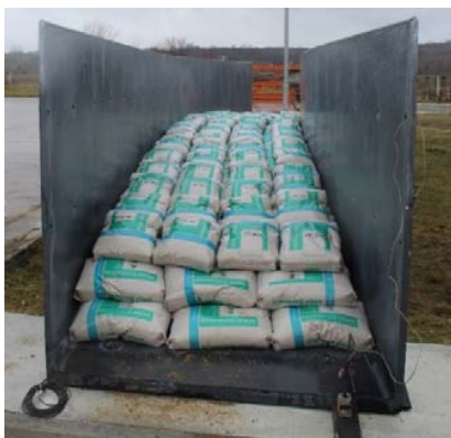
Fig. 15 Perform static loading test on footbridge I
