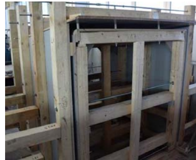
Fig. 8 Formwork of test sample
