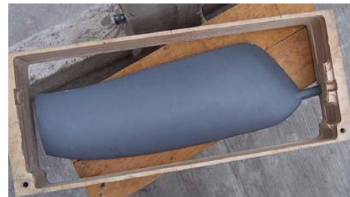
Fig. 13 The polished and varnished blade that was removed from the wood block
