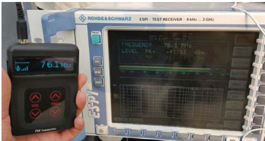
Fig. 9 Implementation result of embedded FM transmission control SW
