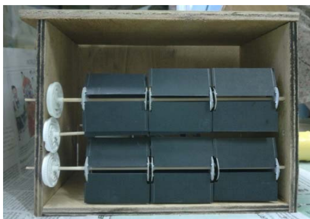
Fig. 3 The front view of the electrical flipping advertisement board
