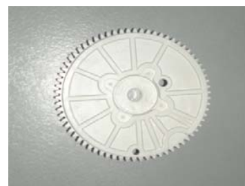
Fig. 2 (a) Plastic, 70 teeth, 3.5cm diameter gear
