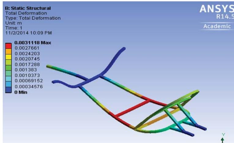
Fig. 9 Total deformation result for Design 6
