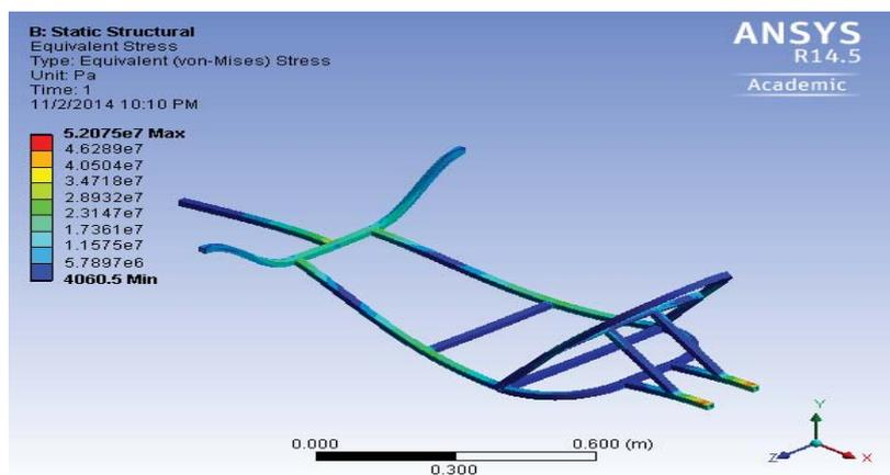
Fig. 11 Von-Mises equivalent stress result for Design 6
