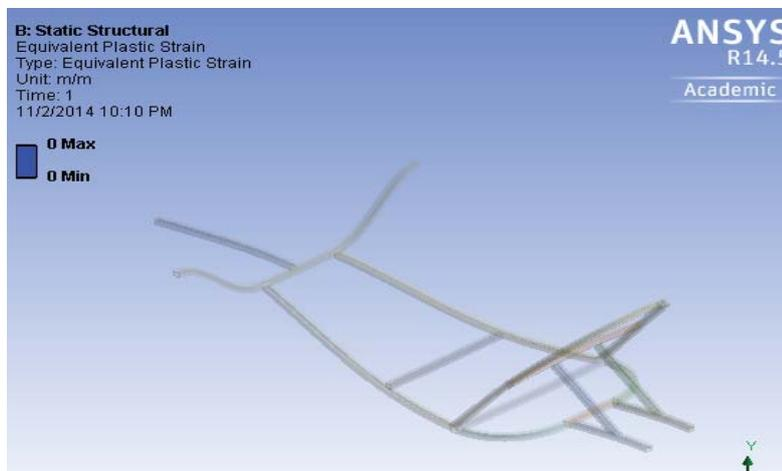
Fig. 10 Plastic deformation result for Design 6
