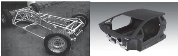
Fig. 3 Triangulated Chassis and Monocoque Chassis
