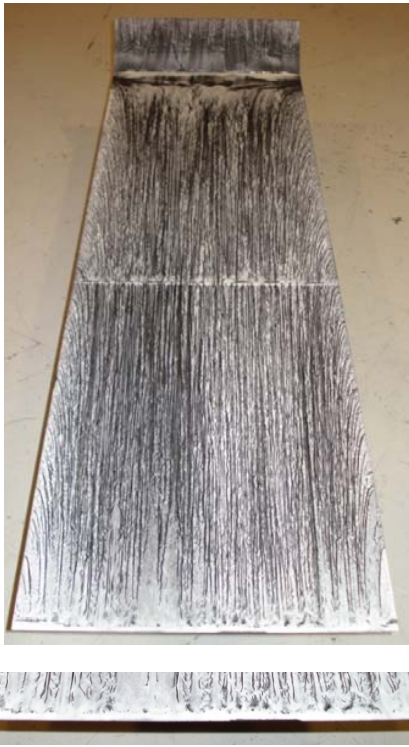
Fig. 5: Flow visualization over the plate with trailing edge flap at 40^\circ . Entire plate and close up of leading edge.
