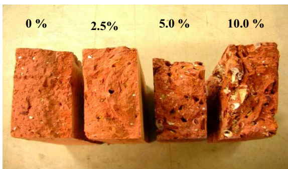
Fig. 3 Cross sections of bricks for mixes with 0 %, 2.5 %, 5 % and 10 % CBs
