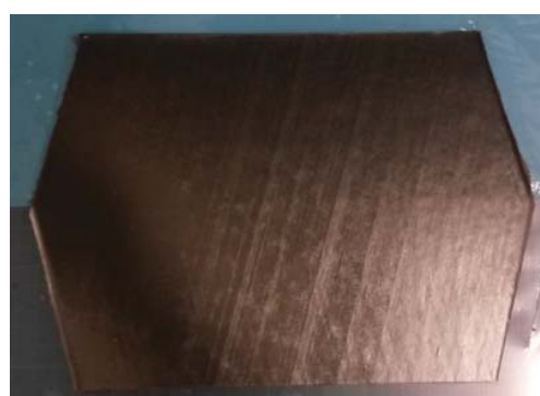
Fig. 9 Flat UD Panel Layup with Film Insert (Panel 6)
