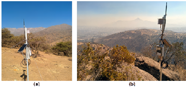
Fig. 7 Two prototype nodes of the wireless sensor network deployed in the Quebrada de Ramón basin for the proposed FFEWS prototype. The skyline of the city of Santiago de Chile can be seen on (b)
