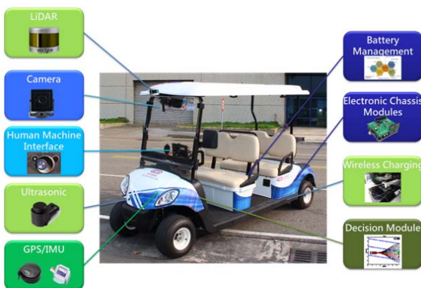
Fig. 8 The in-house built self-driving e-golf cart
