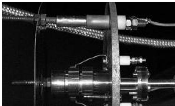
Fig. 4 The hollow cathode heater test platform
