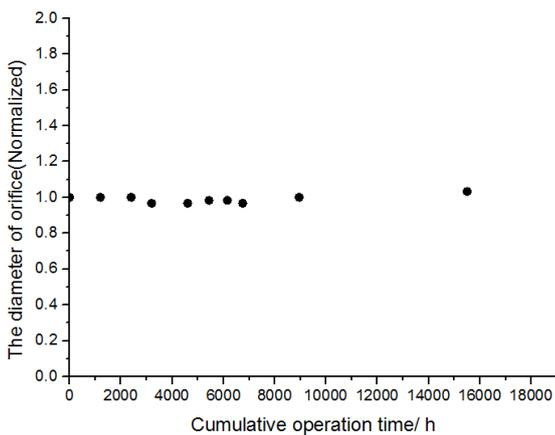
Fig. 7 The diameter of orifice versus operation time
