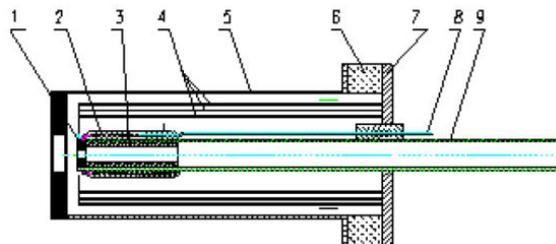
Fig. 1 The schematic of the hollow cathode; 1-the orifice plate, 2-heater, 3-LaB<sub>6</sub> insert, 4-thermal shield, 5-keeper, 6-isolator of ceramic, 7-mounted flange, 8- the cable of heater, 9-tube
