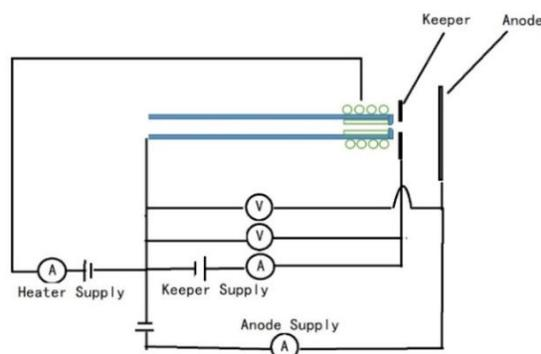
Fig. 3 Test apparatus for discharge cathode life test
